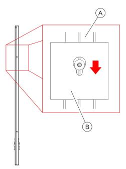
Fit the PDU into the provided fitting slots via the attachment for the existing mounting solution in the rack (Fig. 22).
