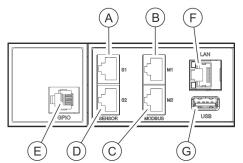
Fig. 3: Connector panel (Master PDU)
