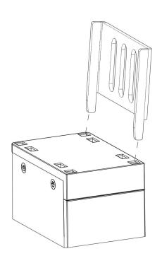
Fig. 19: Fitting the plug-in brackets
