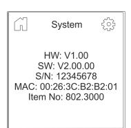
3. View "SW:" to read the software version of the PDU.
