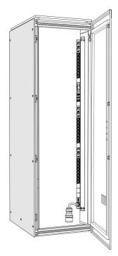
**3.** Fasten the PDU to the rack with screws via both plug-in brackets (Fig. 20).
