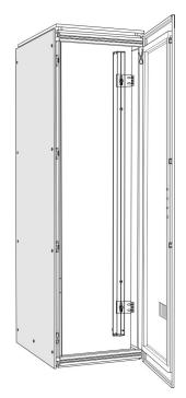
**4.** Fit the PDU onto the mounting brackets (Fig. 16).
