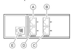
Fig. 4: Connector panel (Slave PDU)
