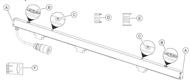
Fig. 6: Overview of the fitting options for the PDU
