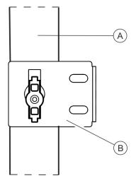
Fig. 14: Installation with mounting brackets
