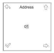
Fig. 30: Setting the Modbus address
