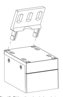
Fig. 17: Fitting the plug-in brackets
