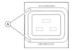
Fig. 11: Status LEDs on the sockets
