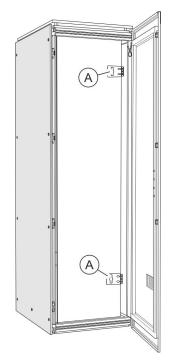
Fig. 15: Rack with mounting brackets
